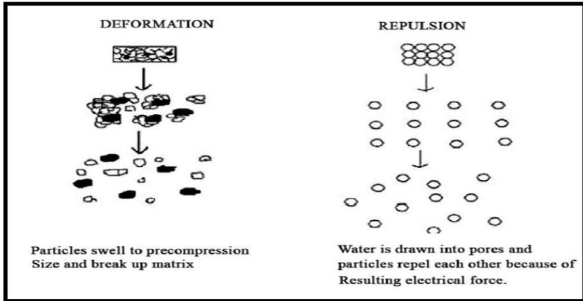
**Figure 2. Mechanism of Superdisintegrant- Deformation & Repulsion**
