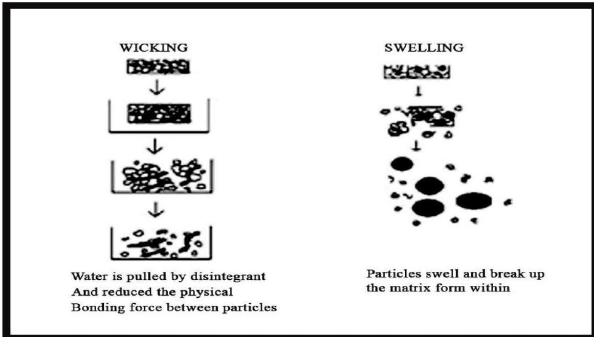
Figure 1. Mechanism of superdisintegrant - wicking & swelling
