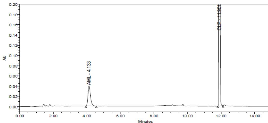
**Figure 2: Chromatogram of tablet dosage form contains 12.5  $\mu$ g/ml of AML and 375  $\mu$ g/ml of CLP (Numlopar tablet contain 2.5mg AML and 75mg CLP)**
