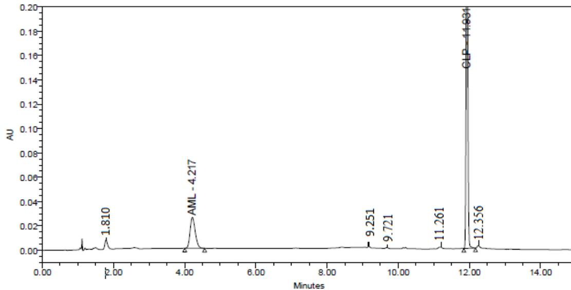
**Figure 3: Chromatogram of acid-treated AML and CLP. Chromatogram of acid (1 N HCl) hydrolyzed AML and CLP showing degradation peaks at retention time (TR) 1.810 min, 9.251 min, 11.261 min, 12.256 min.**
