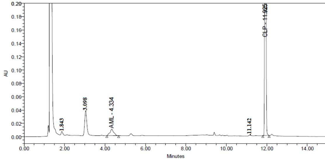
**Figure 5: Chromatogram of H<sub>2</sub>O<sub>2</sub> treated AML and CLP. Chromatogram of chemically oxidized AML and CLP using 3% H<sub>2</sub>O<sub>2</sub> showing degradation peak at T<sub>R</sub> 1.523 min, 1.843 min, 3.098 min, 11.142 min.**
