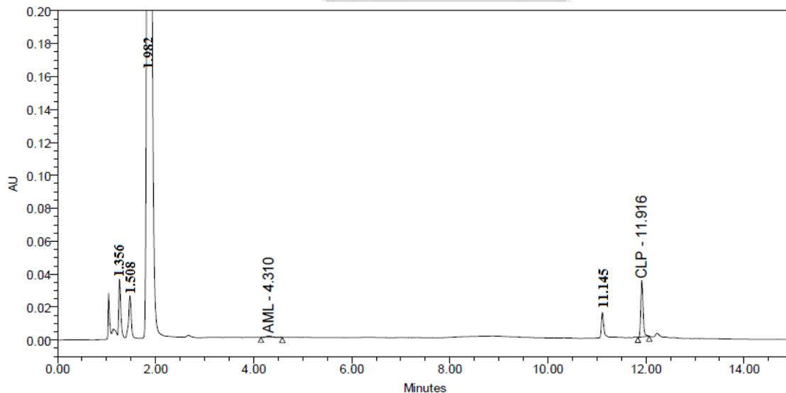
**Figure 4: Chromatogram of base-treated AML and CLP. Chromatogram of base (1 N NaOH) hydrolyzed AML and CLP showing degradation peaks at retention time (TR) 1.356 min, 1.508 min, 1.982 min, 11.145 min.**
