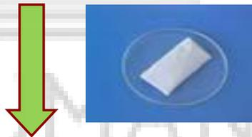
The wrapped sample is then taken out from petroleum ether and is left in a fume hood to remove the solvent.
