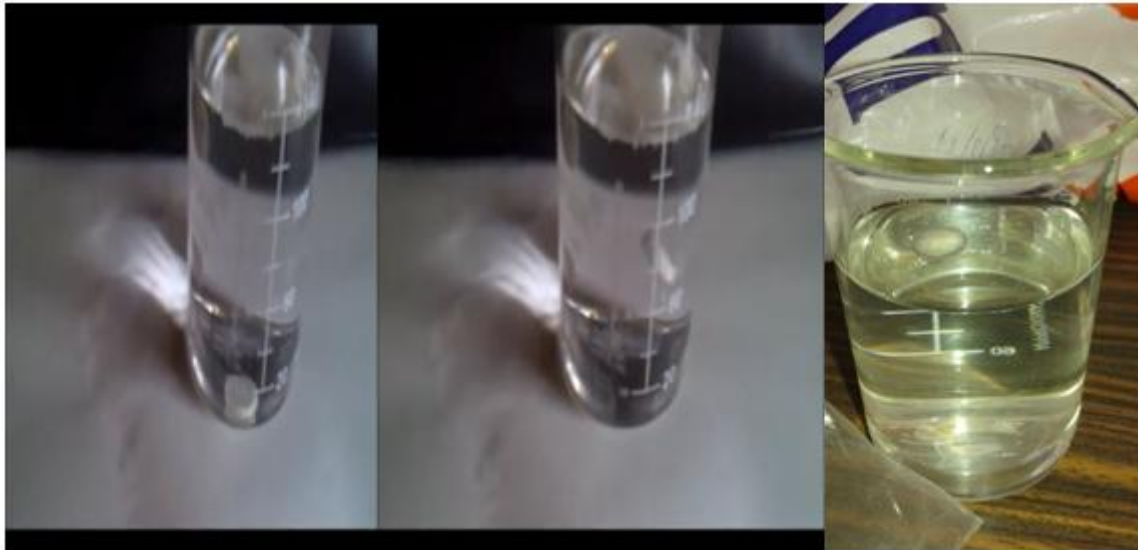
Figure 4: Initial Floating, Float in 16 sec, FLT MT 12hrs.
