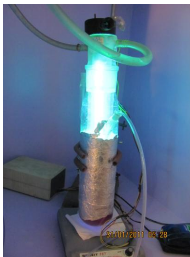
Figure 2. Experimental set up for photocatalytic reaction
