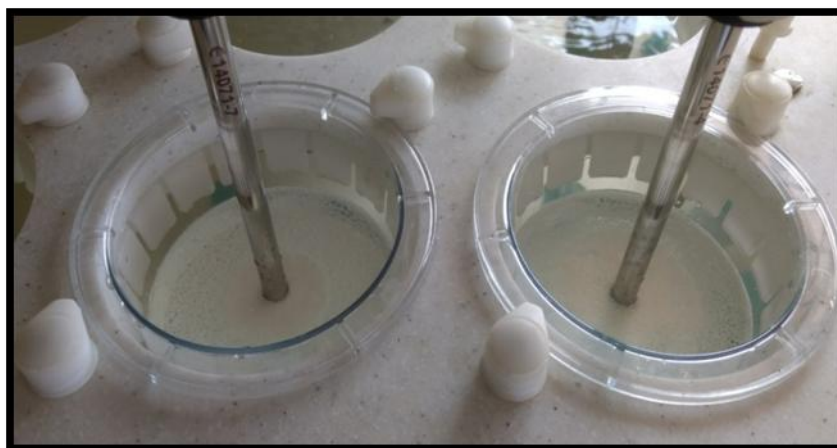
Figure 7: In-vitro dissolution studies using USP type-II apparatus (rotating paddle)
