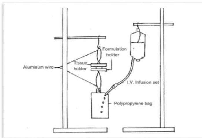
Figure (2): Modified apparatus for *in-vitro* bioadhesion test adopted from (Habib et al., 2010).
