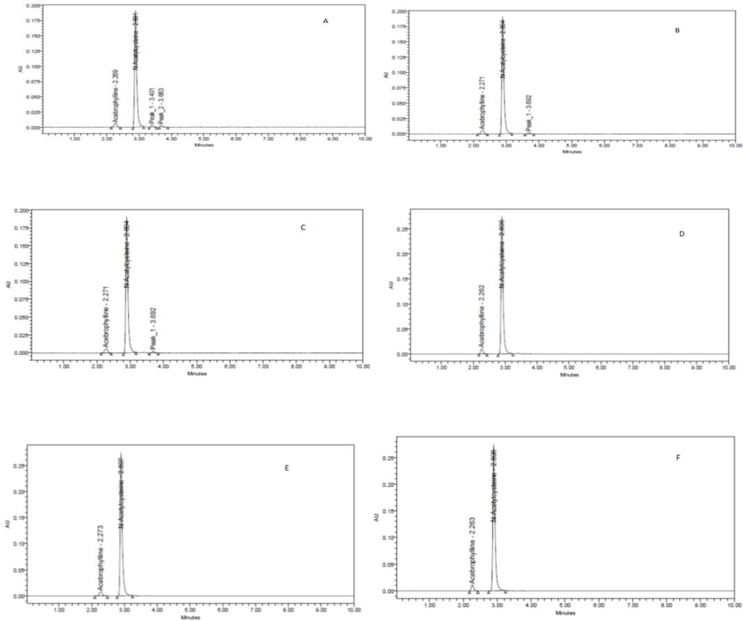
**Figure No. 5: Forced degradation chromatograms of acebrophylline and acetylcysteine (A: Acid degradation, B: Base degradation, C: Peroxide degradation, D: Thermal degradation, E: UV degradation, F: Neutral degradation)**
