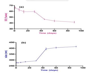
Figure (6): Effect of 3 months storage at 4°C on (a) MXF entrapment efficiency in NLs and (b) Particle size of MXF loaded NLs.
