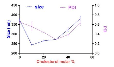
Figure (2): Effect of CH molar percent on PS and PDI of MXF loaded NLs
