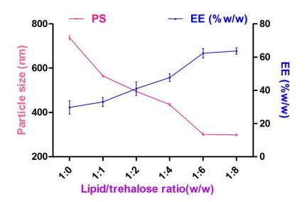
Figure (7): Effect of trehalose mass ratio on the particle size and entrapment efficiency of FDNLs.
