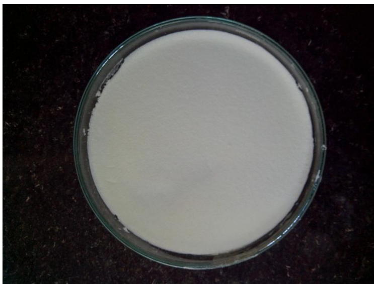
Fig. 1 Image of optimized batch scaffolds prepared by lyophilization
