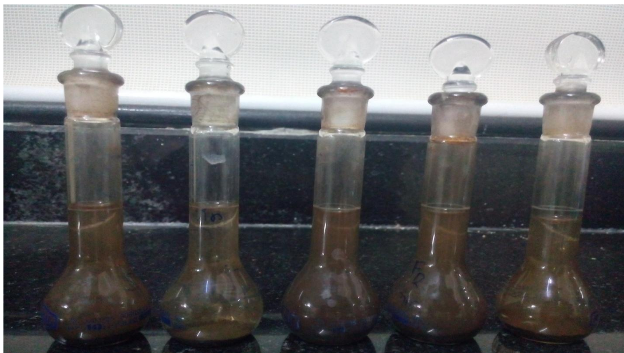
Fig. 3 Synthesis of silver nanoparticle indicated by change in colour
