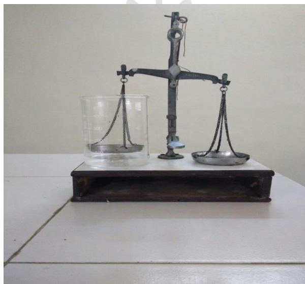
Figure 1: Modified double beam physical balance for in vitro mucoadhesion study
