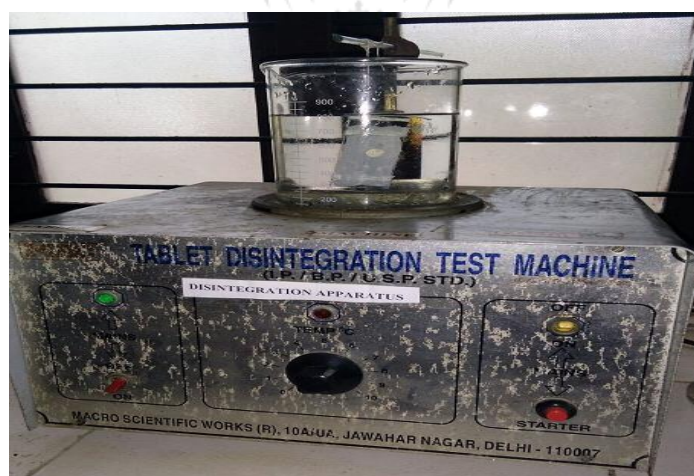
Figure 2: Modified disintegration apparatus
