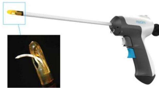
Figure: 2; The tip of the delivery device contains an 18-gauge PEEK needle where 12 small holes allow for water vapor to be circumferentially emitted.
