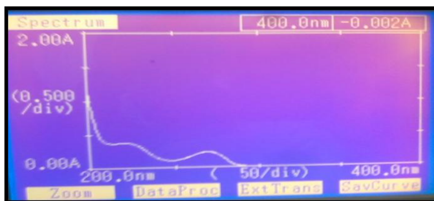
Figure 7: UV spectrum of Pioglitazone HCl in 0.1 N HCl
