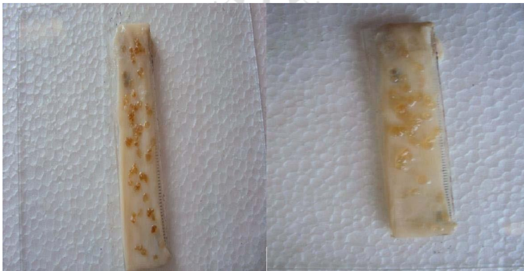
Figure No. 7: Glass side with mucoadhesive microspheres before test and after test
