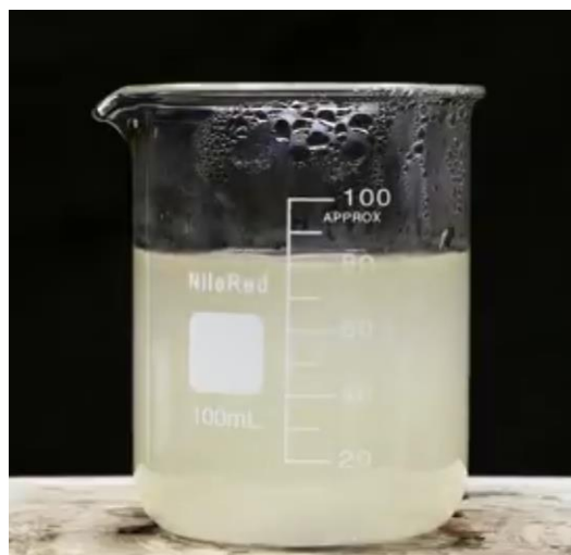
Figure No. 3: Evaporation of tricalcium citrate and development of citric acid crystal
