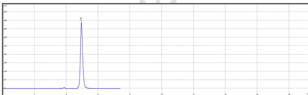
Figure No. 23: Chromatogram of Thermolytic degradation of Dabigatran in Methanol: HPLC Water (90:10 % v/v, pH 3) at flow rate of 0.8 ml/min at 227nm
