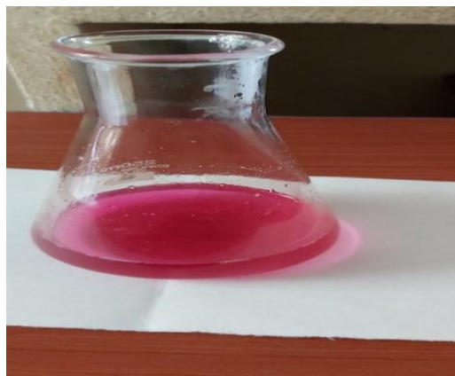
Figure No. 2: Results of test for ANC of test suspension (HCl added)
