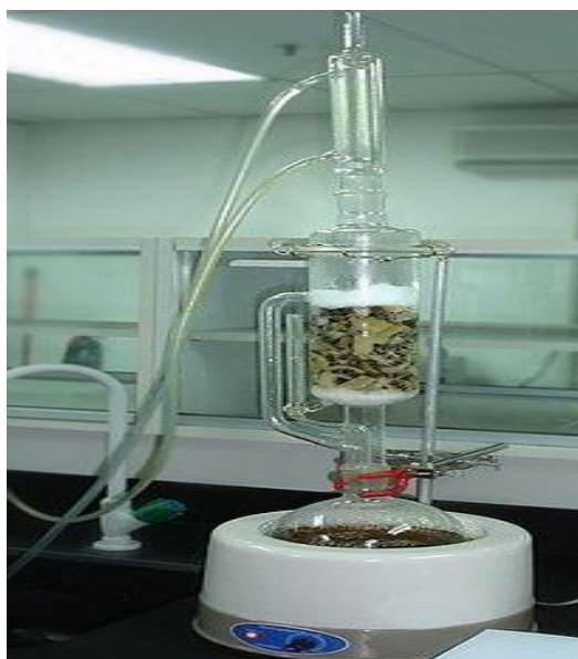
Figure No. 2: A picture of Soxhlet apparatus during an extraction
