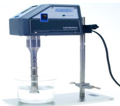
Figure No. 6: Probe Type Ultrasonic Homogenizer
