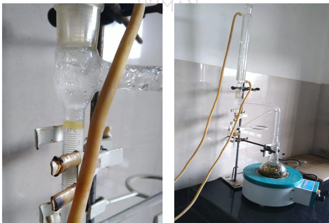
Fig No. 1: Extraction of Lemongrass oil using Clavenger's Apparatus
