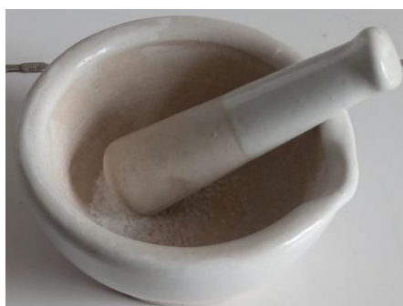
Figure No. 3: Solid-state or Neat grinding Technique.
