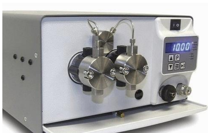
FIG. NO. 3: PUMP SYSTEM IN HPLC
