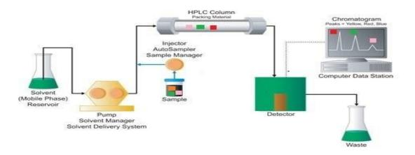
**Figure 1:** Instrumentation of HPLC
