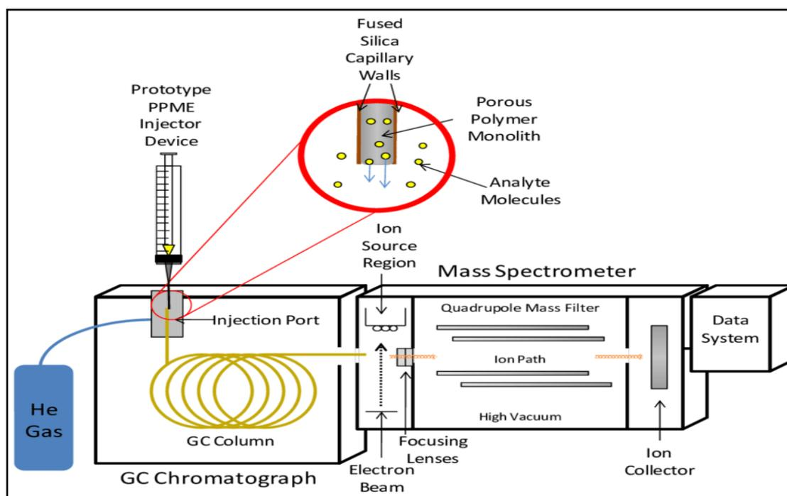
Figure no 1: Schematic of a GC-MS system<sup>[16]</sup>
