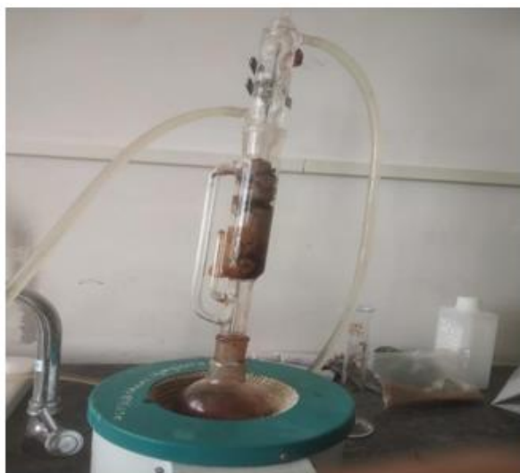
Fig no.4: Soxhlet Apparatus Extraction Method
