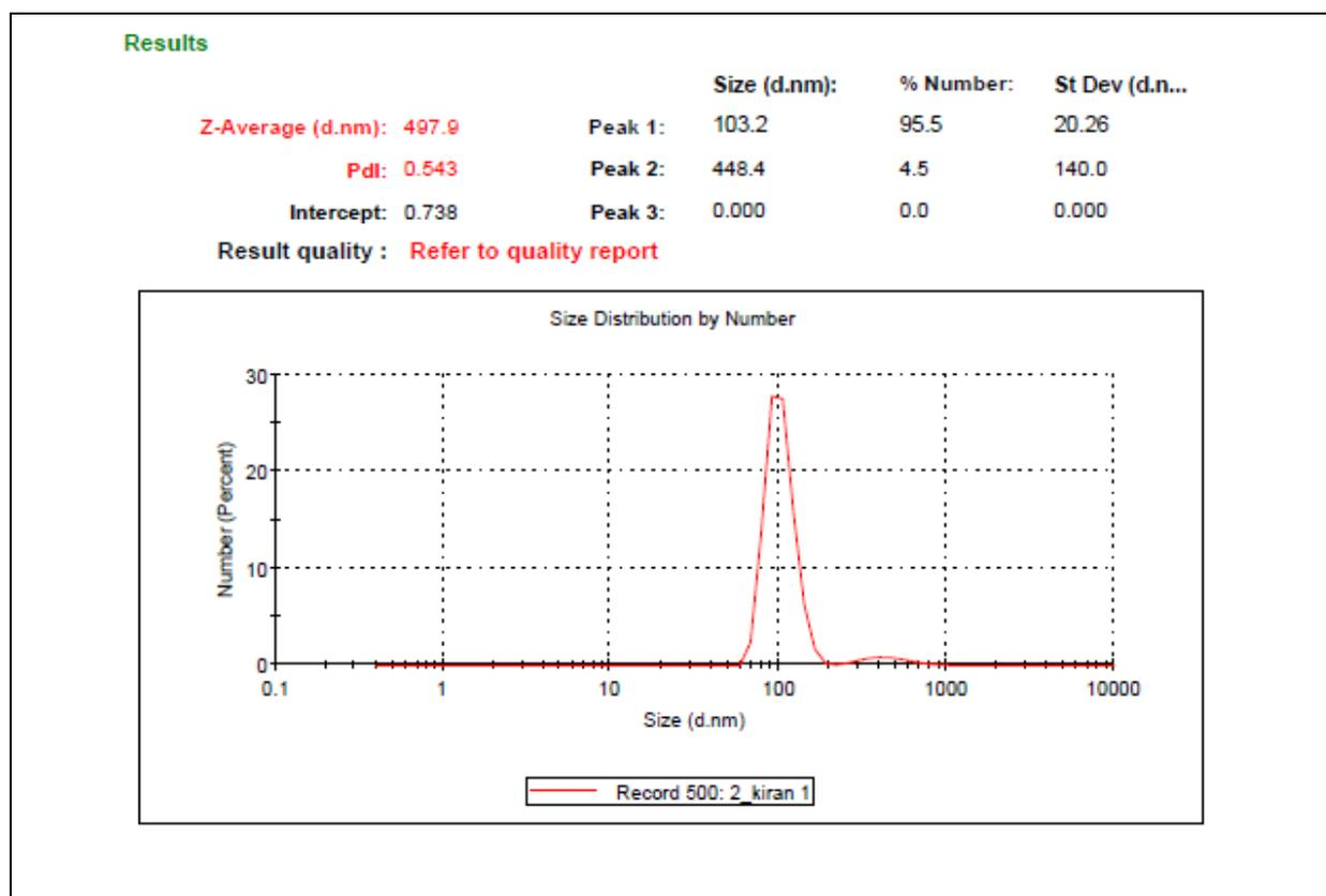
Figure no 4: Particle size analysis of silver nanoparticles.
