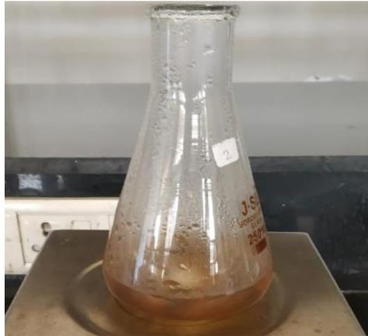
Figure no 2: Colour change that indicates synthesis of silver nanoparticles
