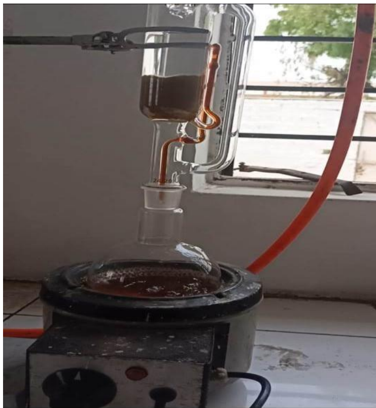
Fig 6: Soxhlet Assembly of Liquorice root Extraction
