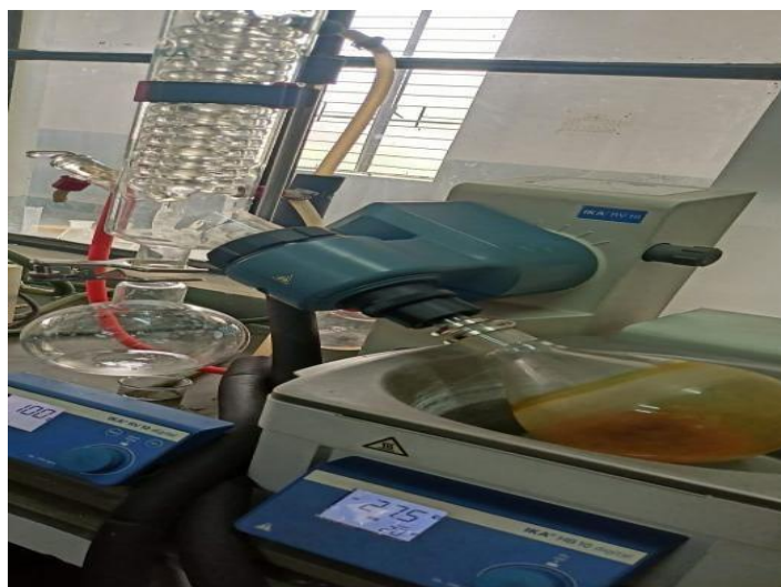
Fig 9: Rota Evaporator with Liquorice Extract
