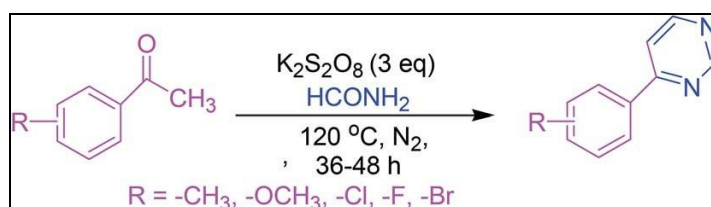
Fig. 5: Synthesis via K 2 S 2 O 8 -facilitated oxidative annulation reaction.
