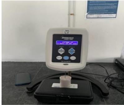
**Fig 3: Brookfield viscometer- viscosity determination**
