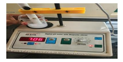
The pH meter was calibrated with the help of a standard buffer solution. Weigh 0.5 gm of cream and dissolved it in 50.0ml of distilled water and its p H was measured with the help of a digital pH meter.
