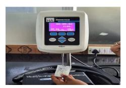
The viscosity of the cream was determined with the help of a Brookfield viscometer at 100 rpm with the spindle no.
