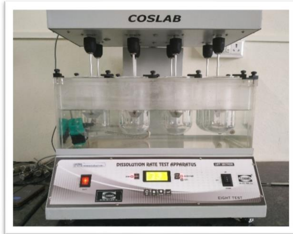
Fig. No. 06: Dissolution of Tablet
