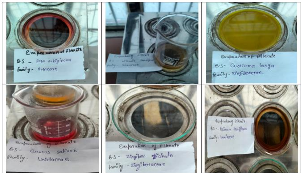
Fig 6: Evaporation of solvent to obtain Solid Extract
