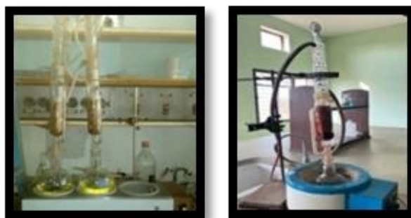
Figure 2: Method of extraction of licorice and Manjistha extract through Soxhlet apparatus
