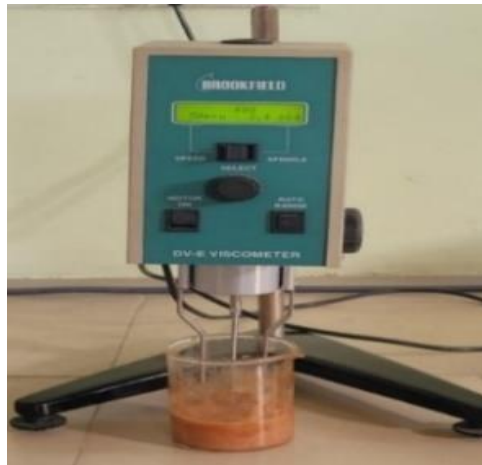
Fig 9: Viscosity determination by the Brookfield viscometer
