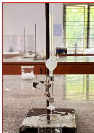
Fig 5: Evaluation of surface tension.
