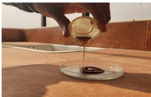
Fig 1.2 method of forming film in the petriplate
