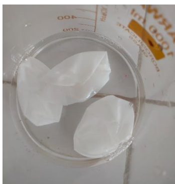
Fig no 1: Decalcified of egg shell In 10% acetic acid
