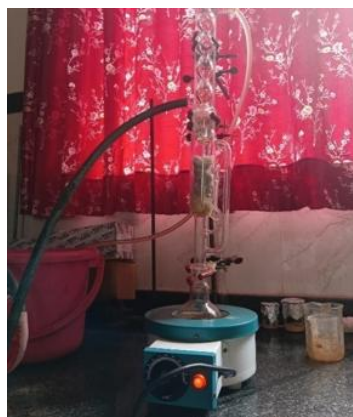
Fig. 2 Experimental Setup of Soxhlet Extractor
